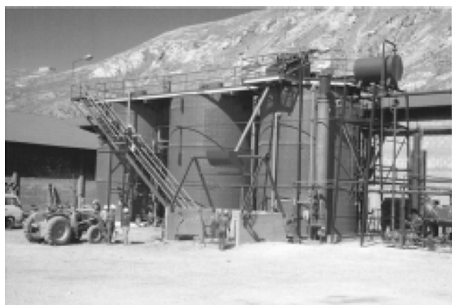
Fig. 4. Heated agitated leaching tanks for iron chloride leaching of silver and lead, Itos, Bolivia. This facility can process treats 15,000 tons of former waste material per month. Plant was erected to treat 1.8 million tons of tin-tungsten tailings containing approximately 400 tons of silver, and large quantities of recoverable antimony, arsenic, lead and copper.
